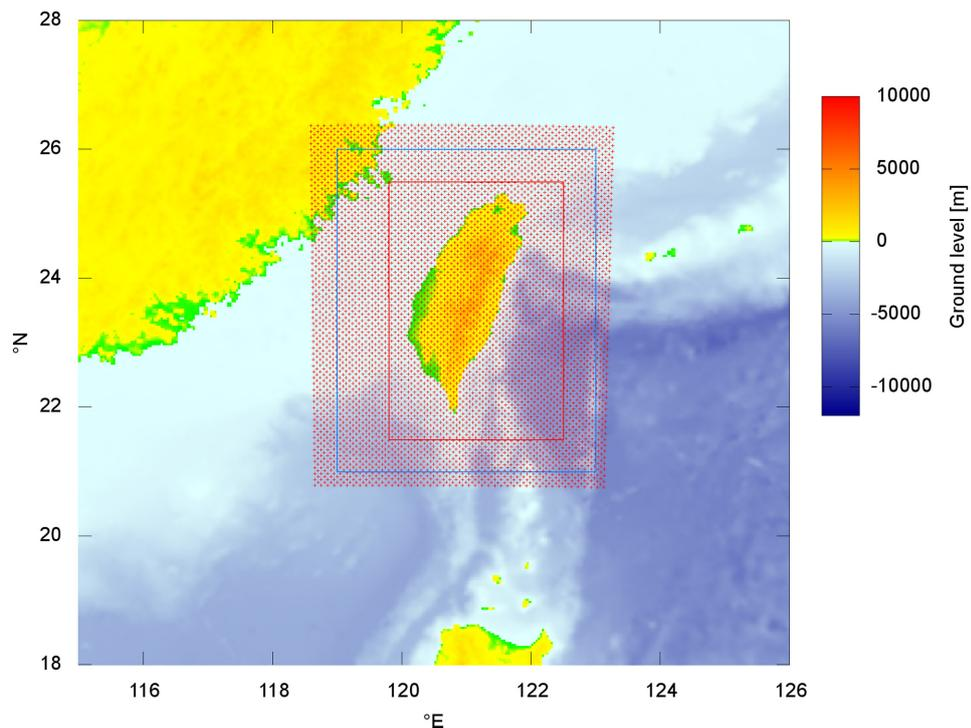
Fig. 3 High resolution wind fields with 5km x 5km resolution (red dots), area of regrided wind-field for simulation (blue box), area of high resolution simulation (red box)
