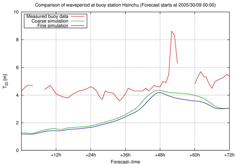
Fig. 10 Comparison of wave periods at Hsinchu
