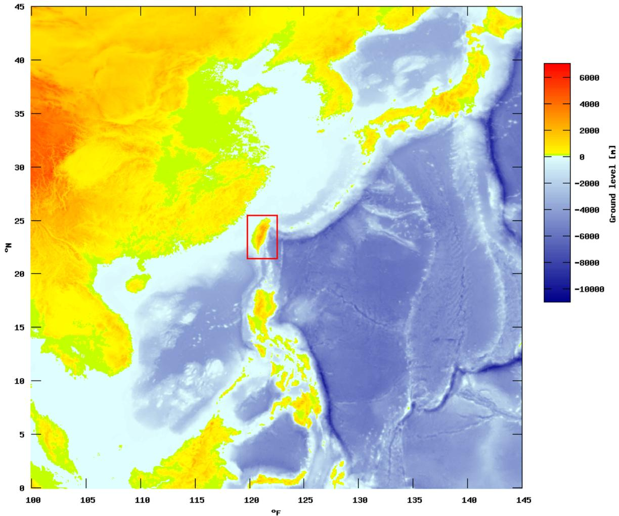
Fig. 4 Bathymetry of area with coarse grid simulation and the nested area for the high resolution simulation (red box)
