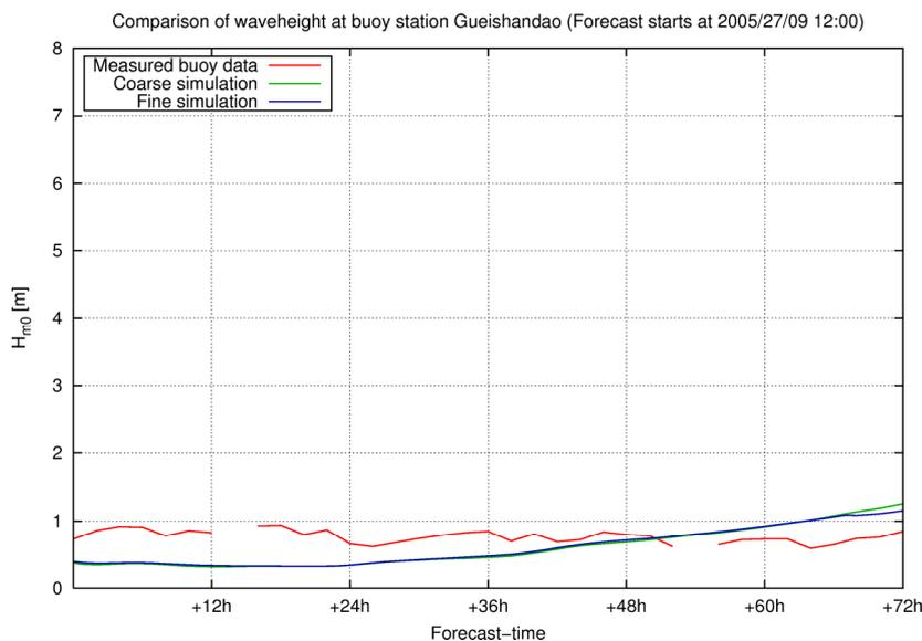
Fig. 6 Comparison of wave heights at Gueishandao
