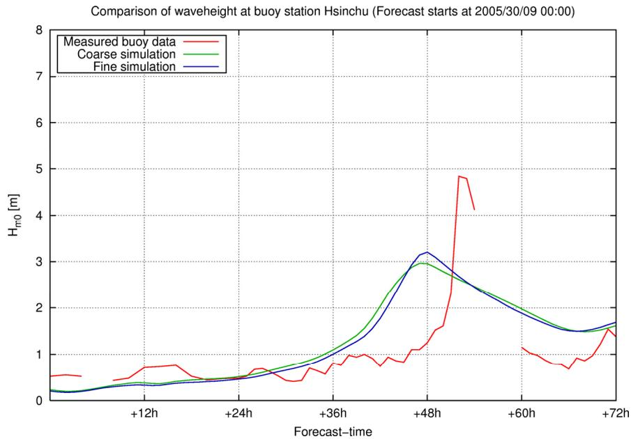
Fig. 9 Comparison of wave heights at Hsinchu
