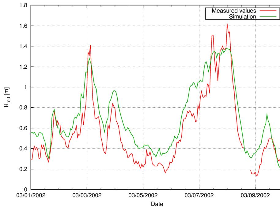
Fig. 11 Example of wave heights from Baltic Sea model at Boergerende
