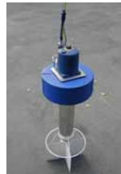
Fig. 5. Drifting GPS buoy
