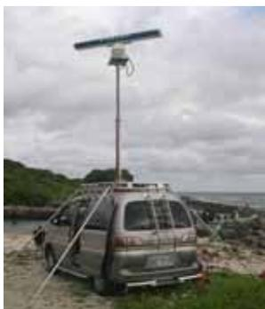
Fig. 3. Mobile marine radar wave and current measurement system
