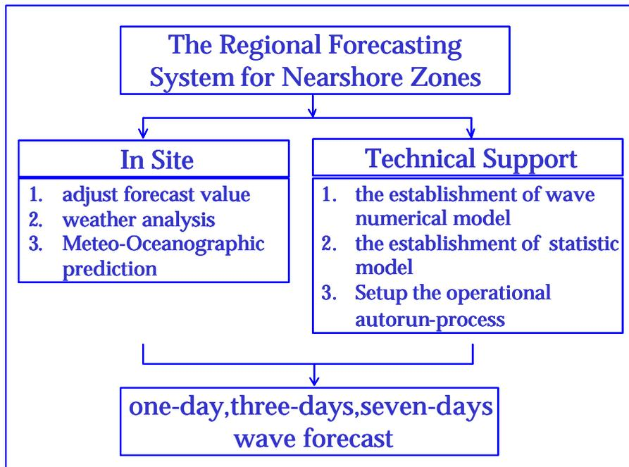
Fig. 2 The operation procedures of the present regional wave forecasting system
