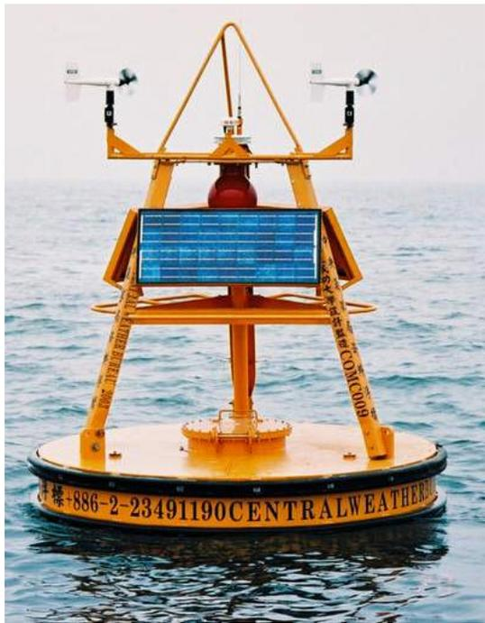
Fig. 2 A photo of marine data buoy (supported by Central Weather Bureau of Taiwan; developed by COMC)
