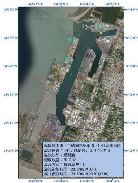
(b) GNOME-simulated drifting trajectory and diffusion range of the fuel oil after 24 hours since the oil spill occurred in the Port of Taichung.
