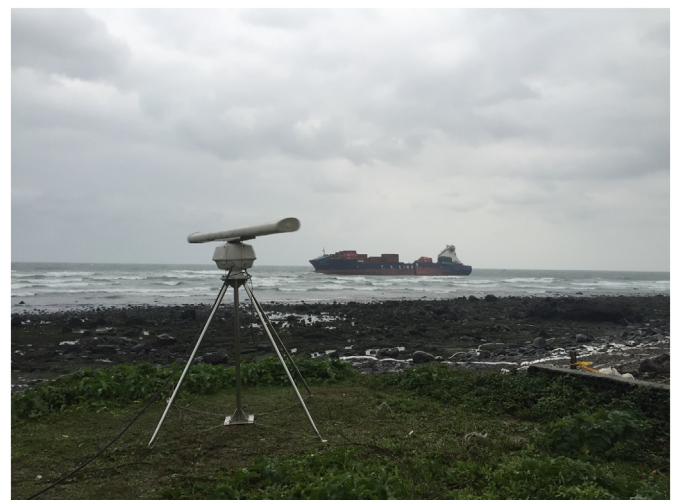
Fig. 4. Setup of an X-band radar at the coast near the container ship T. S. Taipei for monitoring oil spills.
